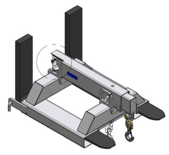
NOTE: All lift truck attachments affect the safe working load of a lift truck. End users should consult their lift truck supplier Fork Arm Retaining Toggles or retaining chain to ensure the lift truck is rated for use with these attachments. In the case of a slung load when lifting a jib attachment, the net lifting capacity should be 0.8 times the rating of the lift truck to allow for the swinging load. Please consult your local lift truck dealer
